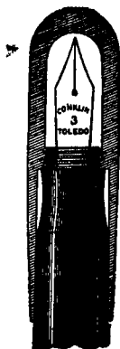
Sectional view of pocket non-leakable pen, showing shoulder in cap abutting against shoulder on pen section, forming air-tight chamber in cap.
