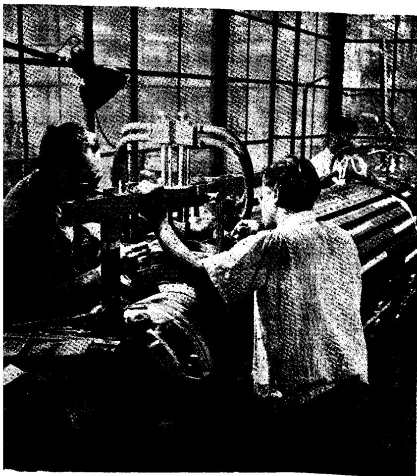
The tank of a giant transformer being fabricated. BELOW : Rotor of a 30 MW turbo generator under construction.
