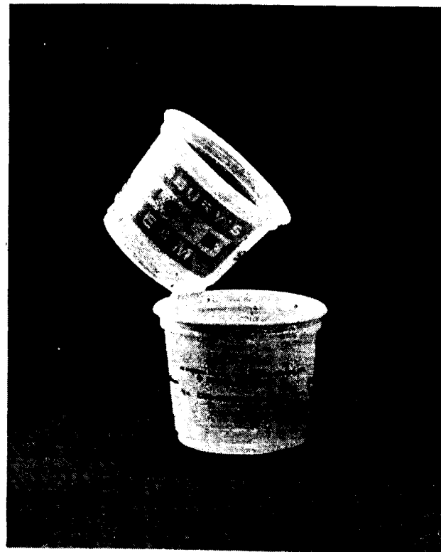
An example of sidewall printing. Note the clearness of the printing.
