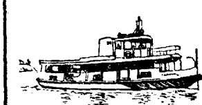
PADMA—the twin screw diesel harbour launch, built for the Commissioners for the Port of Calcutta.
