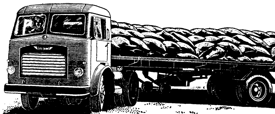
Ashok Leyland Comet 118" wheelbase tractor and Mahindra Owen's "Gama" semi-trailer combination unit
