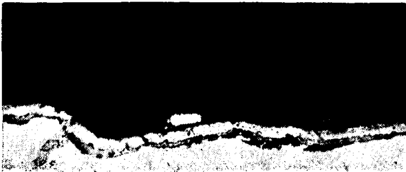
Fig. 13—C-1035 steel. "Green" rod, as-reeled. 500X.
