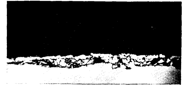
Fig. 23—Tire wire rod, 0.77 C, normal reeling at 1530 F. \text{Fe}_3\text{O}_4 layer thicker and more continuous than in Fig. 22. 500X.
