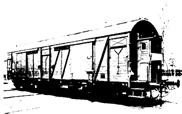
Multiple-purpose wagon for loose and piece goods.
