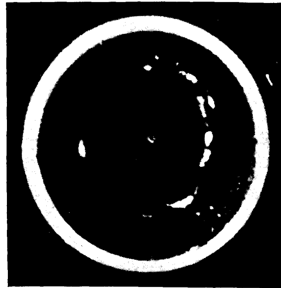
Fig. 4. Rotary section image of a hydronalium roller of 160 mm dia. with defects.
