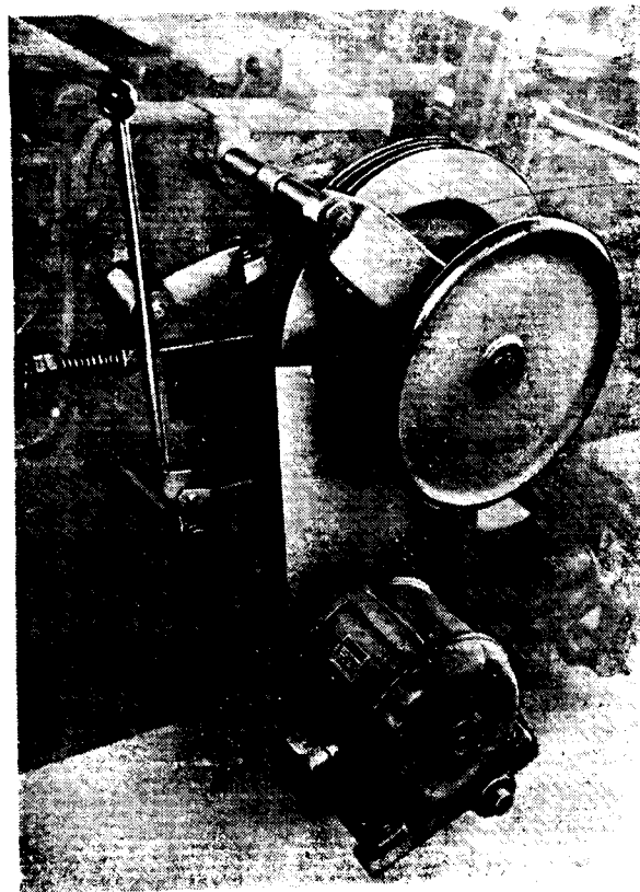
Fig. 5. The sufficiently sized friction clutch and the efficient brake allow high loom speeds. The starting lever at the rear simplifies attendance.
