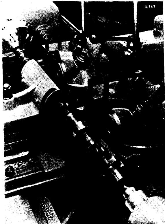
Copying of cams of a Diesel engine camshaft with 2 hydraulic copying slides.
