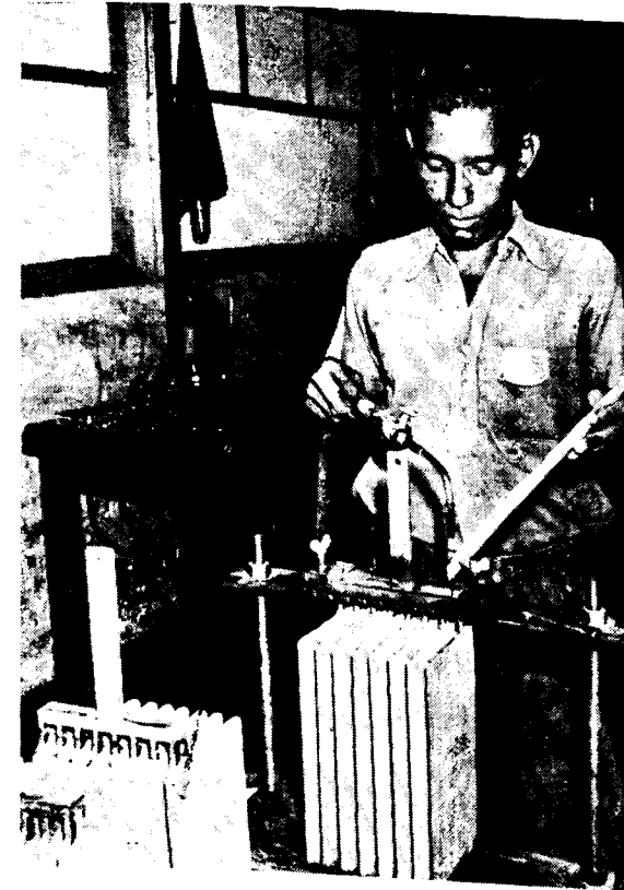
A view of the Pg Section. Assembly of negative plate group.
