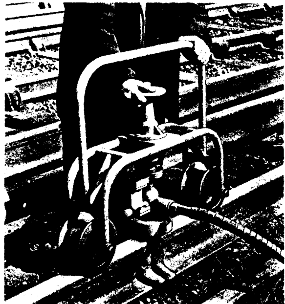
Above: DRILLING a rail ( 1\frac{1}{4} " hole in under two minutes). The under-rail fitting enables the drilling of tracks in use, without impeding the traffic.
