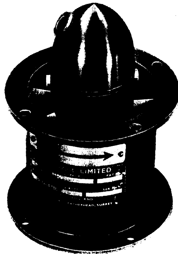
A 2PL81-135 axial blower unit operating from a 400 C.P.S. supply and giving an air displacement of 35 C.F.M. at .85" W.G. This unit weighs only 12 ozs. and is tropicalised for either airborne or ground use.
