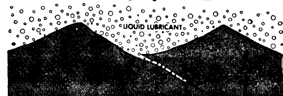
Figure 12. Influence of liquids on progressing hairline crack. Due to capillary action and pressure, liquids enter the cracks and tend to widen and break them.
