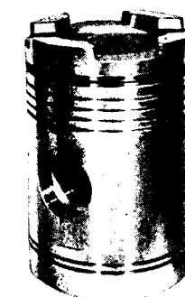
Piston with cast-in ring carrier and cooling device 12 1/4" bore = 317,50 mm.
