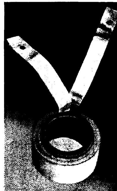
Fig. 4.—Experimental anodised foil winding of 100 turns made from material 1½ in. wide by 0.006 in. thick.
