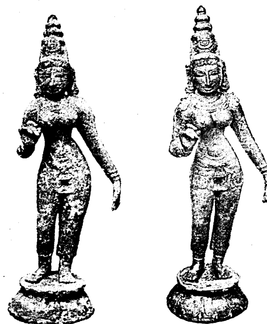
At the Government Museum, bronze images are cleaned through an electrolytic process which is very effective. These pictures show a bronze image before (left) and after such treatment (right).
