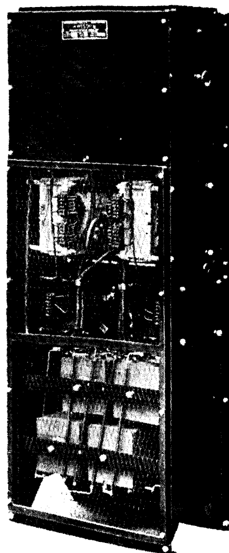
1.2 kW constant voltage charger supplied to Southern Railway. This consists of two 600 watt Westat equipments in series, operating from 220/250 volt 75 c.p.s. single-phase. Output 20 amperes to charge a 480 A.H. battery.
