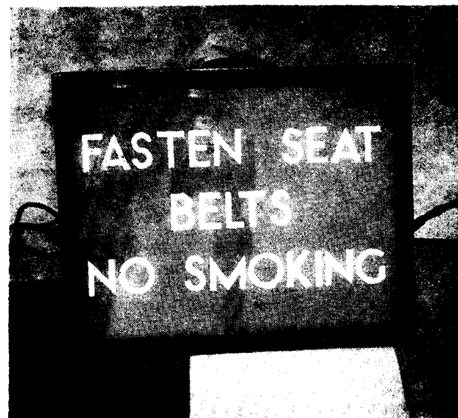
1. An experimental sign plate using an electroluminescent light source. The structure of the plate is similar to that described in Figure 1b of H. K. Henisch's article; zinc sulphide phosphor, shaped electrodes. Excitation at 300 volts and 400 c/s. (The experimental unit was made available through the courtesy of Dr S. T. Henderson of Thorn Electrical Industries Ltd.)
