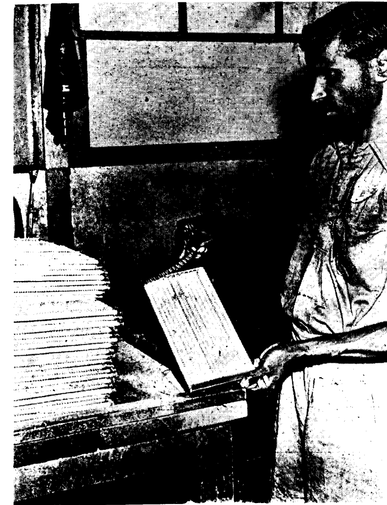
A view of the Pg Battery Section. The positive plates are provided with grit protectors attached by rubber strings
