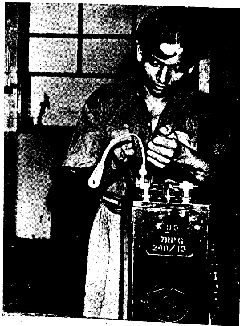
The intercell connecting wires are fitted and the Pg cell is now complete
