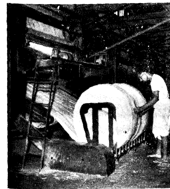
Jute being fed into a carding machine
