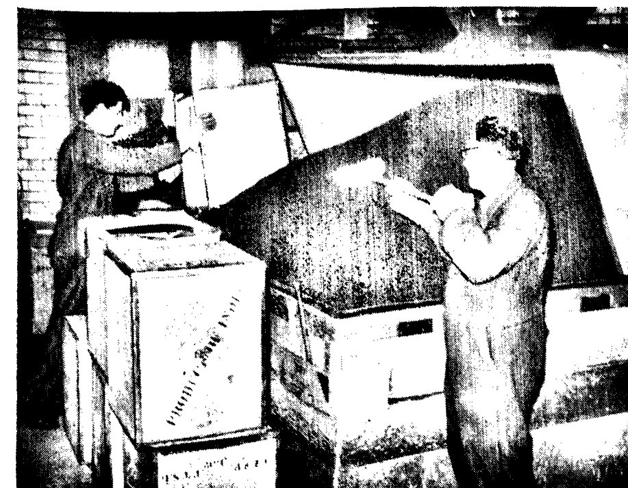
Filling the hopper, leading to the 4,000-lb blending drum
