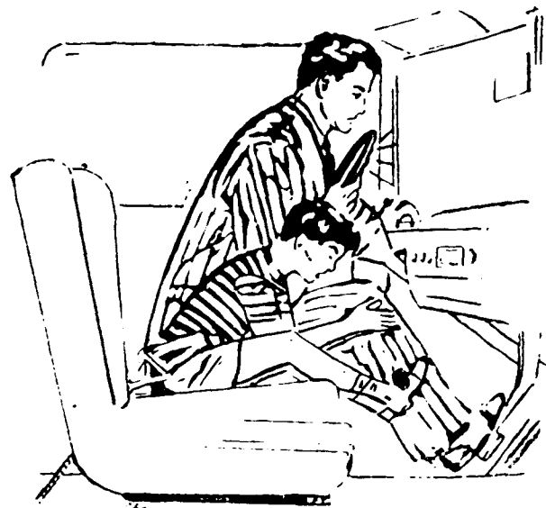
WITH belt, driver and passenger are held in place at moment of crash stop, preventing head blows and greatly reducing chest impact on the wheel.
