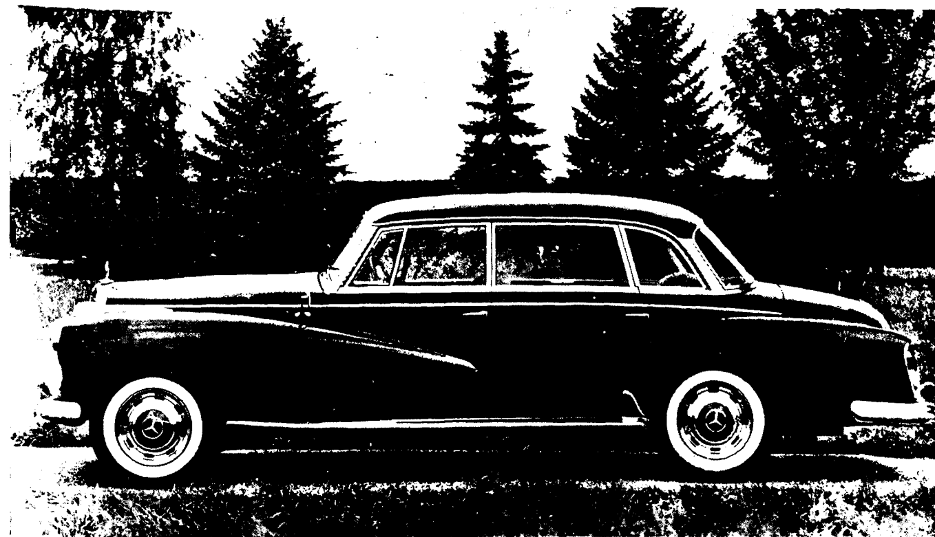
Mercedes Benz 300 automatic with new body and 180 h.p. fuel injection engine
