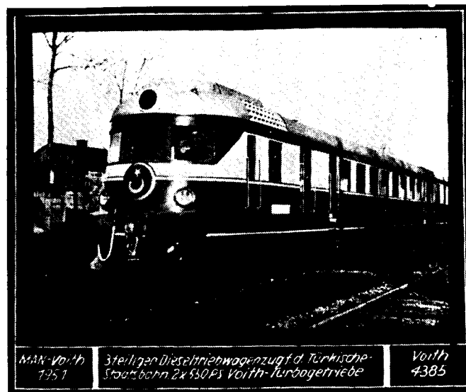
1100 HP. triple articulated Diesel train for the Turkish State Railway (2 engines, 2 Voith Transmissions)
