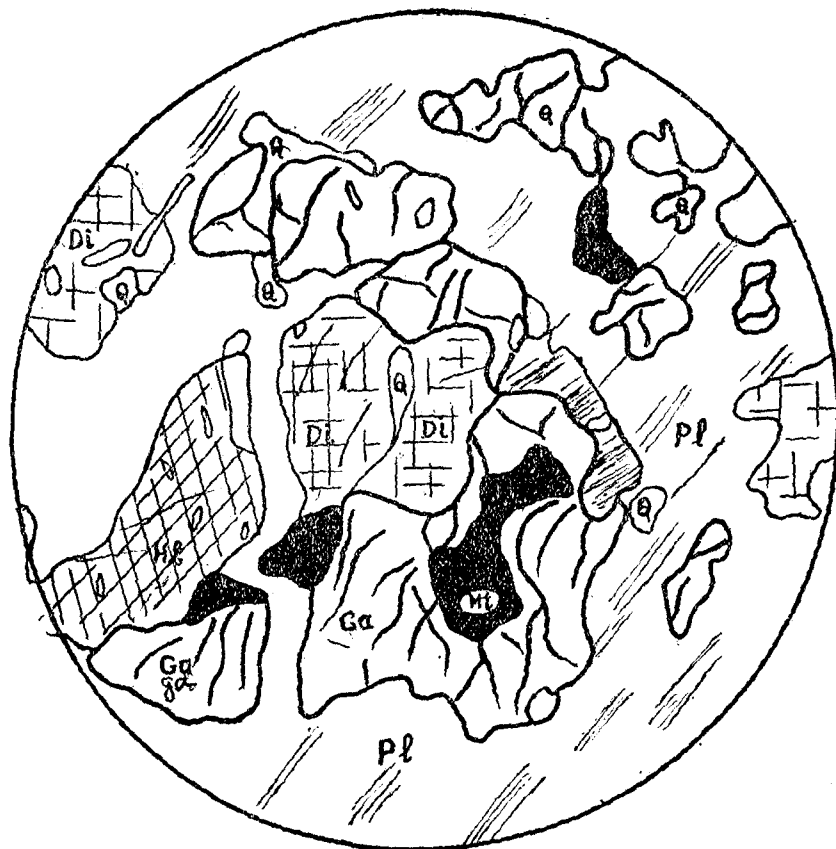
SKETCH 4: Diopside grains are fringed by garnet around the edges. They are also developed around grains of iron-ore.
