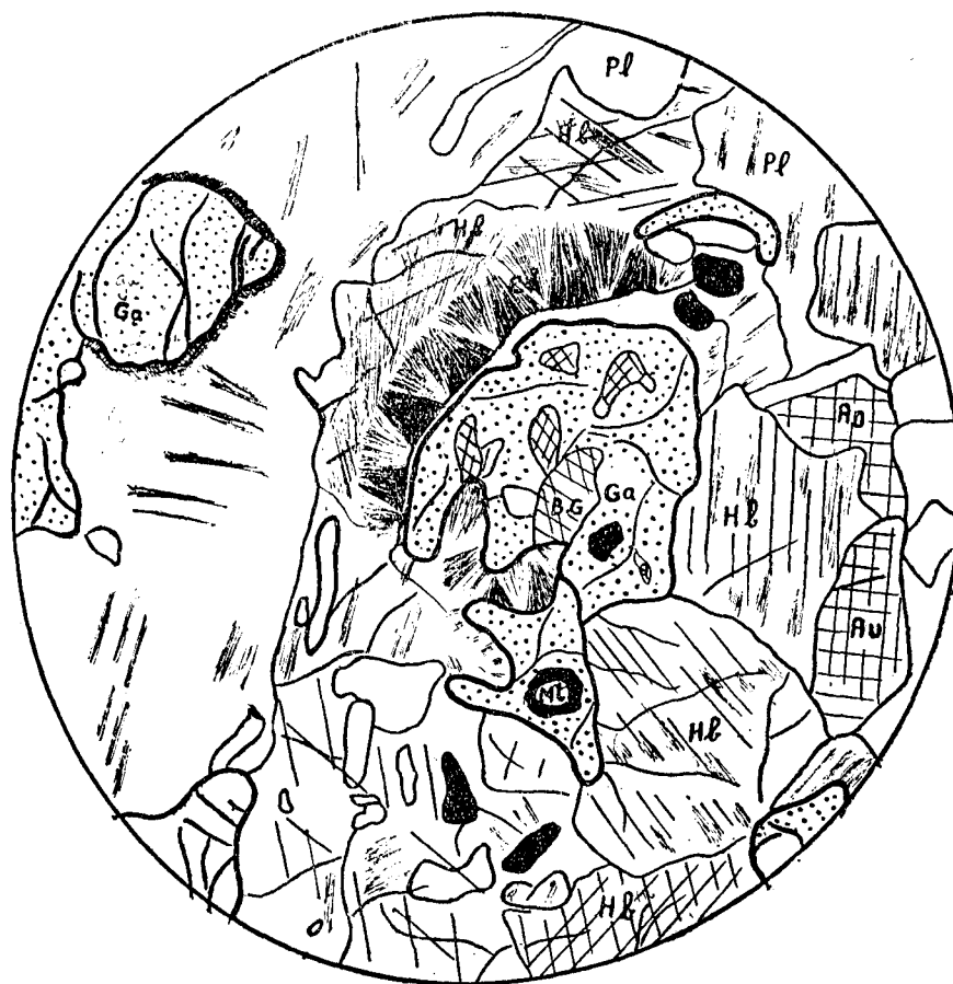
SKETCH 2: Garnet grains are surrounded by a rim of chlorite passing on to hornblende. Blue green hornblende passes into garnet and develops freely. Ga—Garnet. Au—Augite. B.G.—Blue green hornblende. Hb—Hornblende. Ch—Chlorite. Pl—Plagioclase. Mt—Magnetite.
