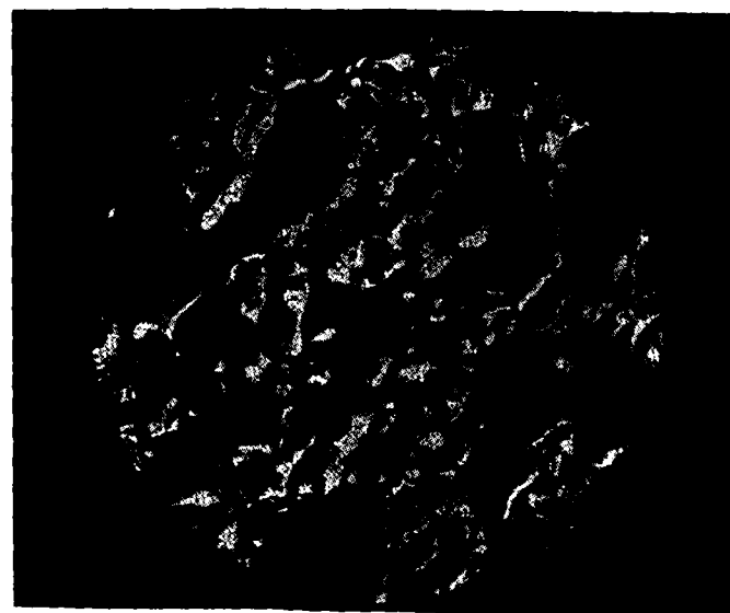
Fig. 6. Photomicrograph of typical Faxfilm replica of a grinding wheel surface when crush dressed.
