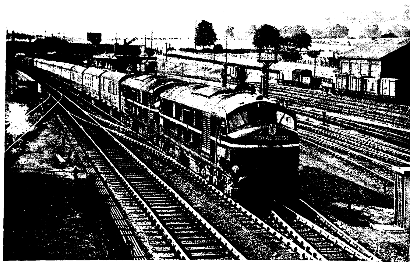
Diesel-electric locomotives Nos. 10000 and 10001. These locomotives, which are in experimental service on British Railways, are seen here hauling the "Royal Scot" heavy express. Each locomotive has a 16 cylinder diesel engine developing 1,600 h.p. Both were built at the Derby Works of British Railways and are equipped with diesel-electric generators made by the English Electric Co.
