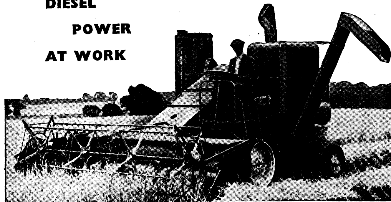
On the farm Perkins Diesel engines offer greater power, easier starting, greatly reduced fuel and maintenance cost. This is a Massey-Harris 780 Combine Harvester fitted with a Perkins L4 TA type diesel engine.
