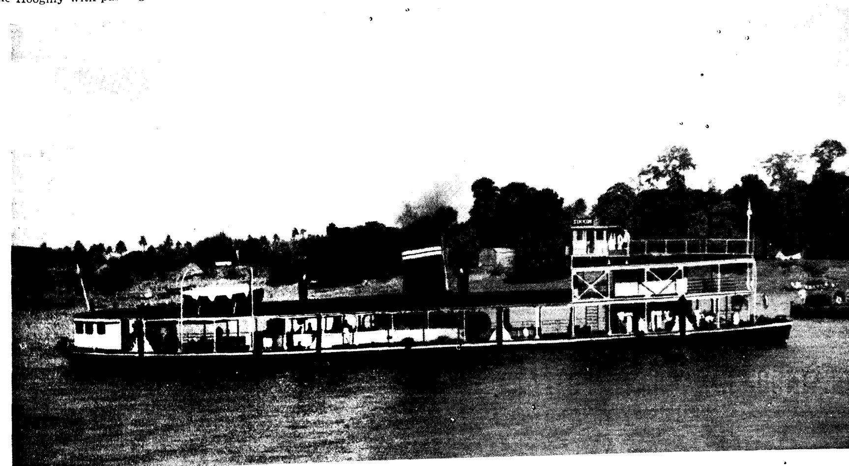
"Sikkim", fitted with modern Kortz nozzles, is a screw tug towing barges and flats
