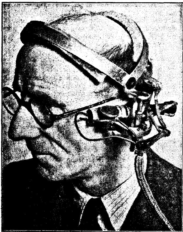
Fig. 2.—Goldie's anoxia meter. The apparatus is lightly clamped to the ear and the oxygen content of the blood is measured by means of two photoelectric cells. (Air Ministry Crown copyright.)
