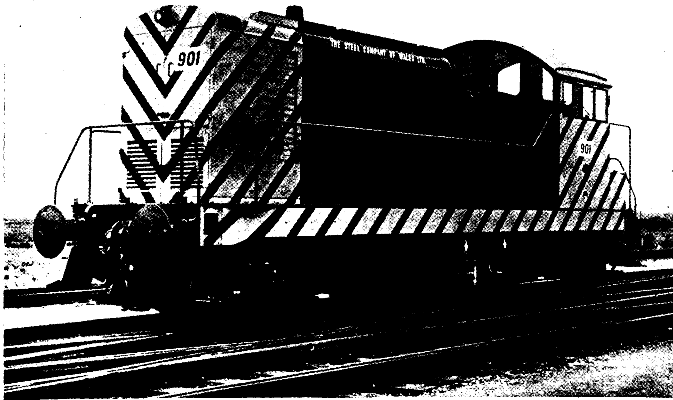
Close-up view of the Brush-Bagnall 515 H. P. Bo. Bo. Locomotive.
