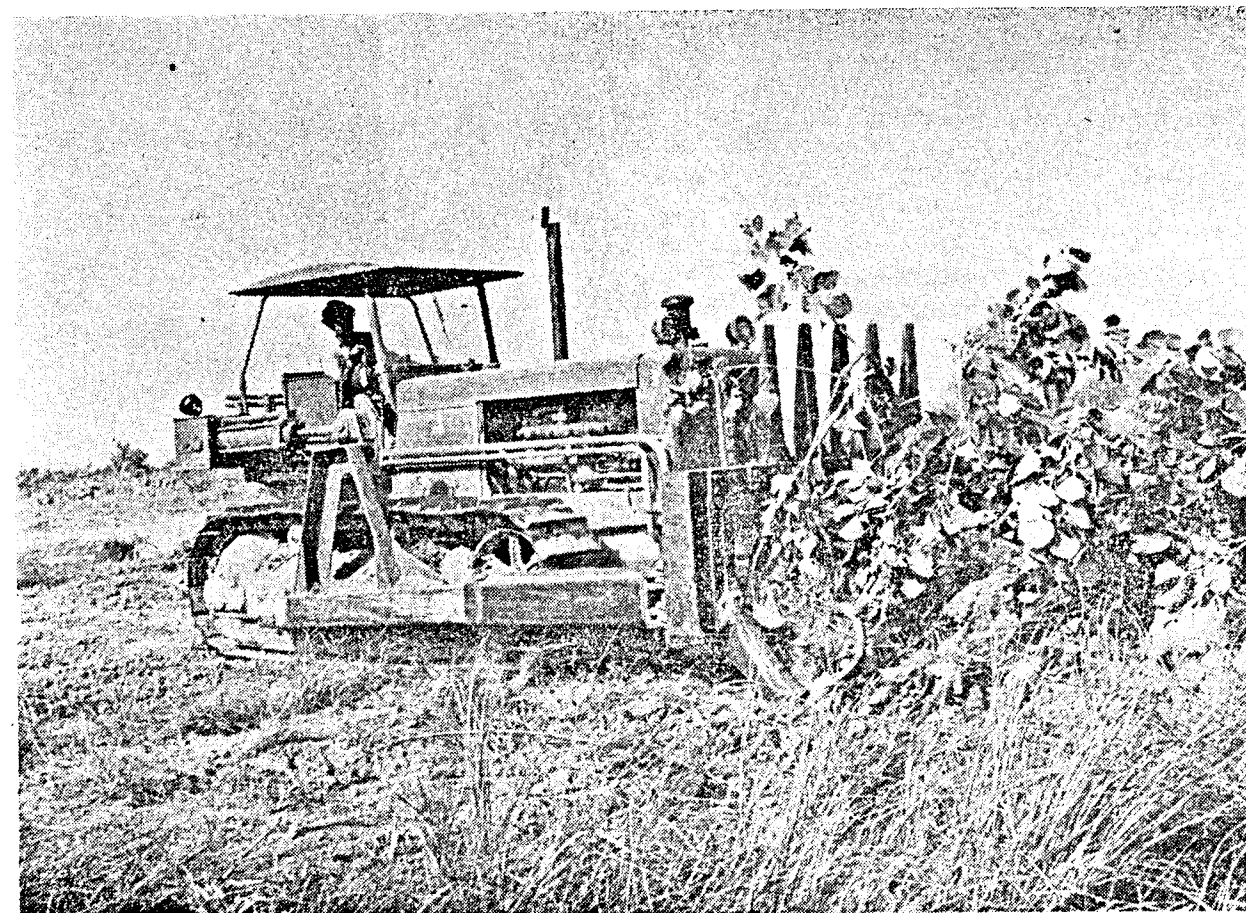
A 'Hanomag' K.90 equipped with root-raker ripping up jungle.
