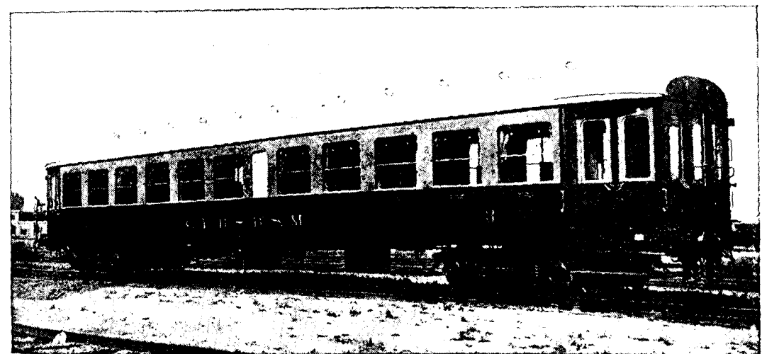
Belgian Railways All-Steel Passenger Coach utilized in long distance services centred on Brussels
