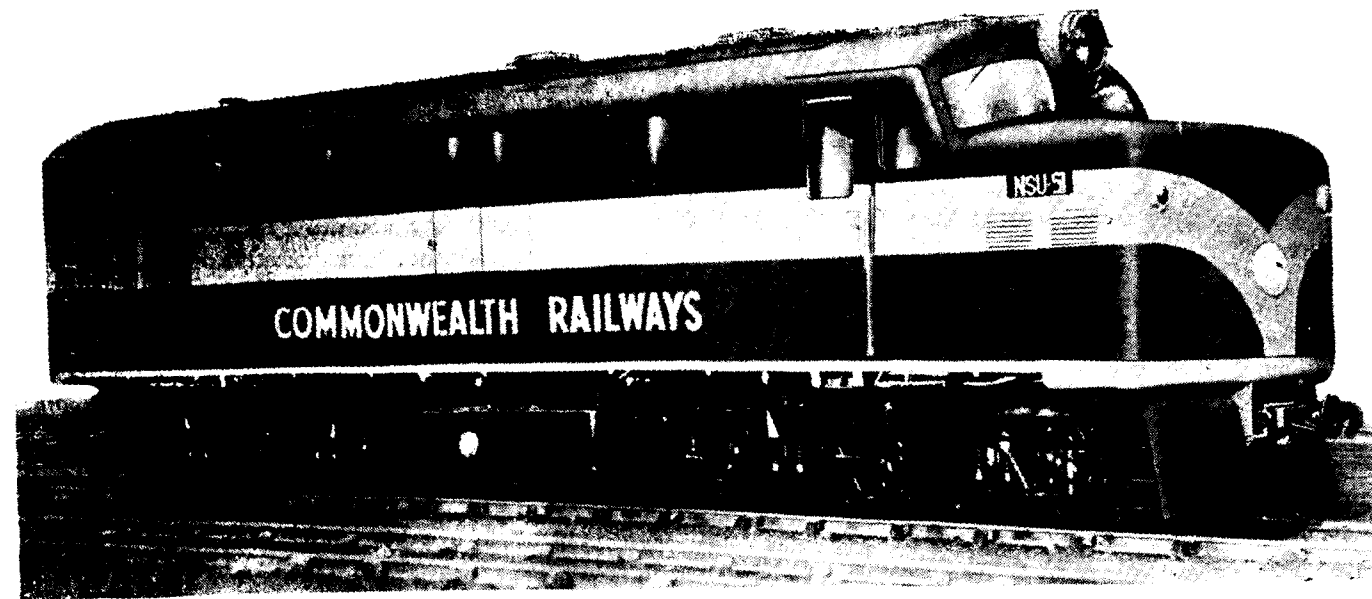
955 b.h.p. ALA-ALA 3 ft. 6 in. gauge diesel-electric locomotive of 62½ tons weight and 50 m.p.h. top speed for the Commonwealth Railways of Australia built by the Birmingham Railway Carriage & Wagon Co. Ltd.
