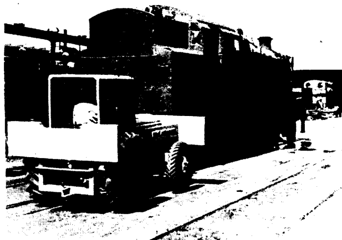
The Epping Auto-Shunter has no difficulty in moving this tank locomotive up a 1 in 30 gradient into the repair shop.
