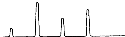
Fig. 2. Portion of a typical mass spectrum, as it might be traced on a rotating drum recorder. The mass/charge ratio of the ions is measured along the horizontal axis, and the peak ion current vertically.
