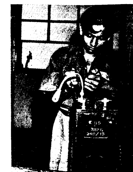
Intercall connecting wires are fitted and the RPg cell (railway battery) is complete.
