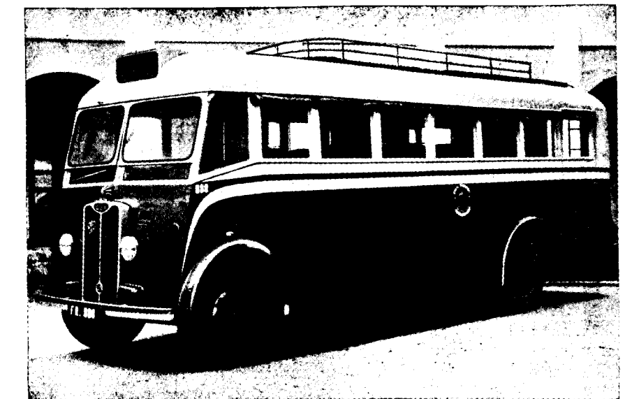
Bus with Alum. Body built for Travancore Cochin State Transport.
