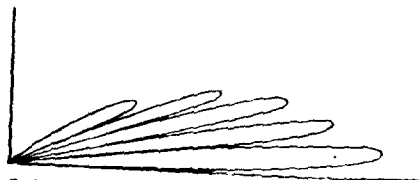
Fig. 9. Polar diagram of sea-reflection radio interferometer.
