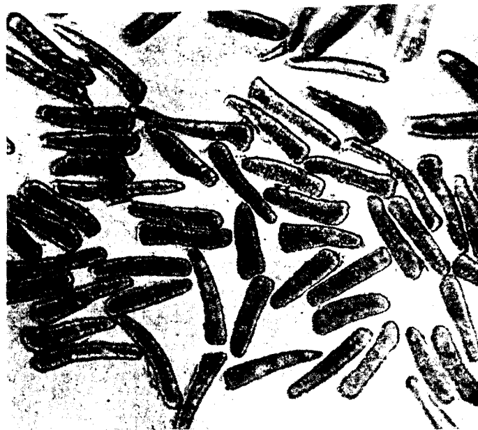
20. Silk, tussah: in cross-section, mounted in gelatine. Magnification \times 500 .
