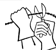
Cable cut — Alarm automatically sounded.
