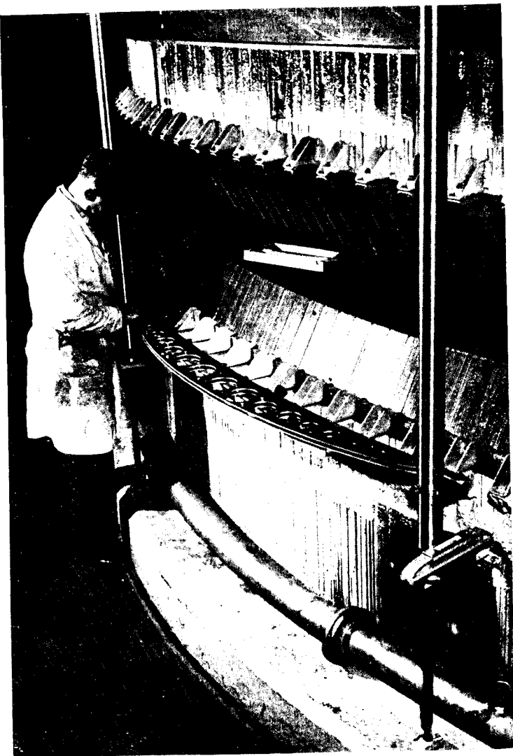
11. Birmingham University, proton synchrotron: showing the laminated construction of the magnet. There are 2,400 laminations, each \frac{1}{2} -inch thick, welded together. (This and the previous two photographs are from the Central Office of Information, Crown Copyright reserved.)
