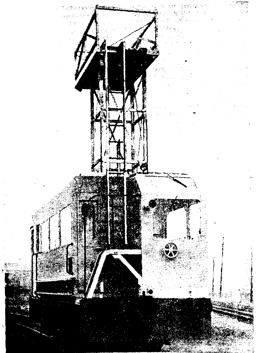
Diesel inspection Car by Drewry Car Co., Ltd., for inspecting overhead line equipment on electrified sections of British Railways.
