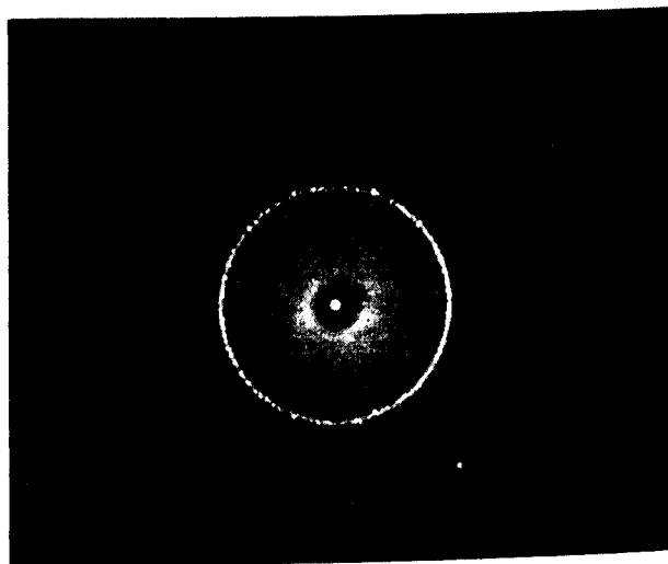
1. Powder photograph of coarsely powdered calcite, using copper X-radiation and a flat film.
