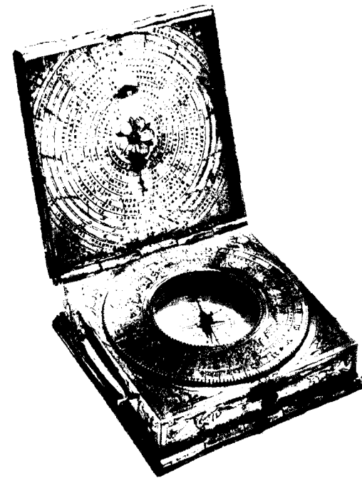
21. Another gift portable instrument, this time including compass, sundials, quadrant and calendar, made by Tobias Volekmer (1645). There is another lid on the bottom of the box, which thus has all six outside surfaces engraved (see below).
