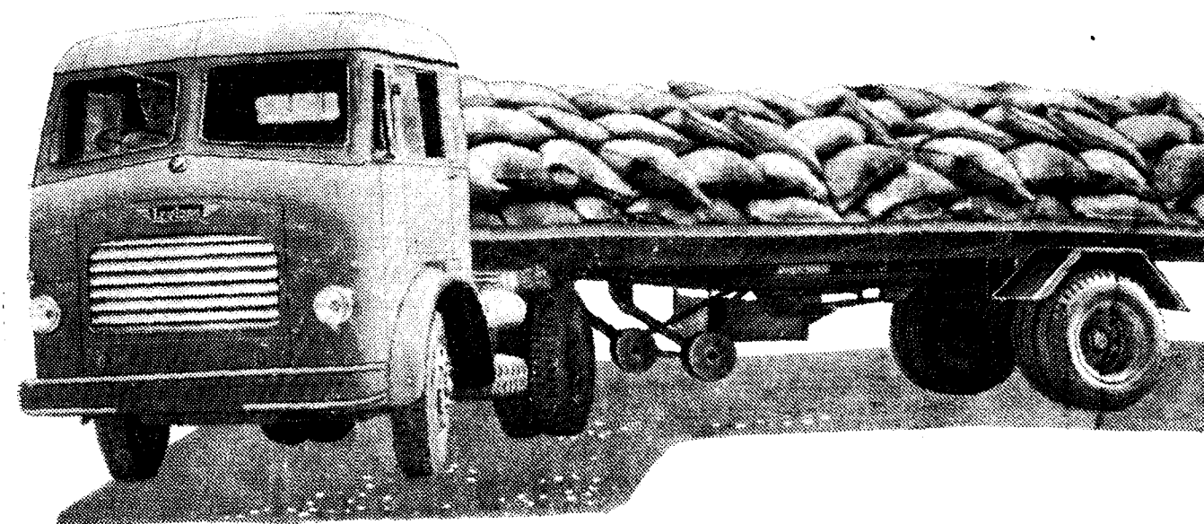
Ashok Leyland Comet 118' wheelbase tractor and Mahindra Owen's "Gama" semi-trailer combination unit.
