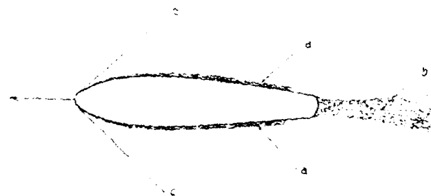
Figure 1—Sources of resistance on a moving body : (a) boundary layer (skin friction); (b) wake (eddy formation); (c) shock waves (wave resistance). Shock waves may also form at other points on the body.
