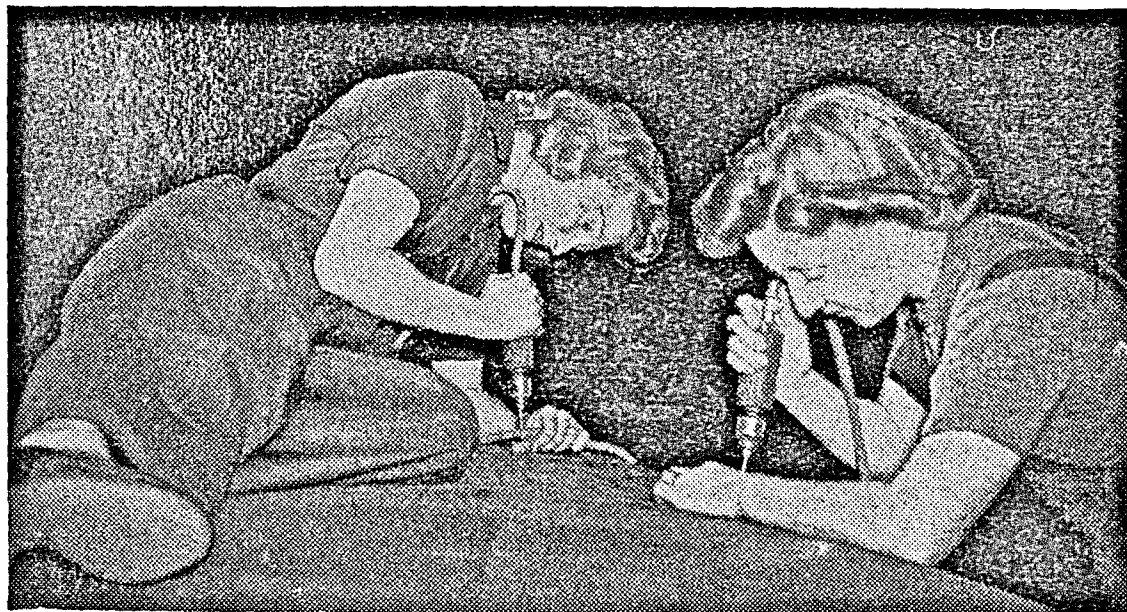
The manufacture of British heavy bombers has been and will continue to be greatly stepped up to carry out intensified R.A.F. bombing raids into the heart of Germany. Picture shows: Women aircraft workers drilling rivet holes in the wing of a "Halifax" four-engined heavy bomber. The "Halifax" weighs 27 tons when fully loaded, carries 5½ tons of bombs, and has a range of 3,000 miles. It has a strong defensive armament of eight Browning machine guns.
