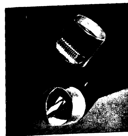
FIGURE 6 Typical Illustration of Transparent Synthetic Resin Mounting (Illustration and half-tone kindly lent by Mr. Adolph I. Buehler, Chicago, Illinois.)
