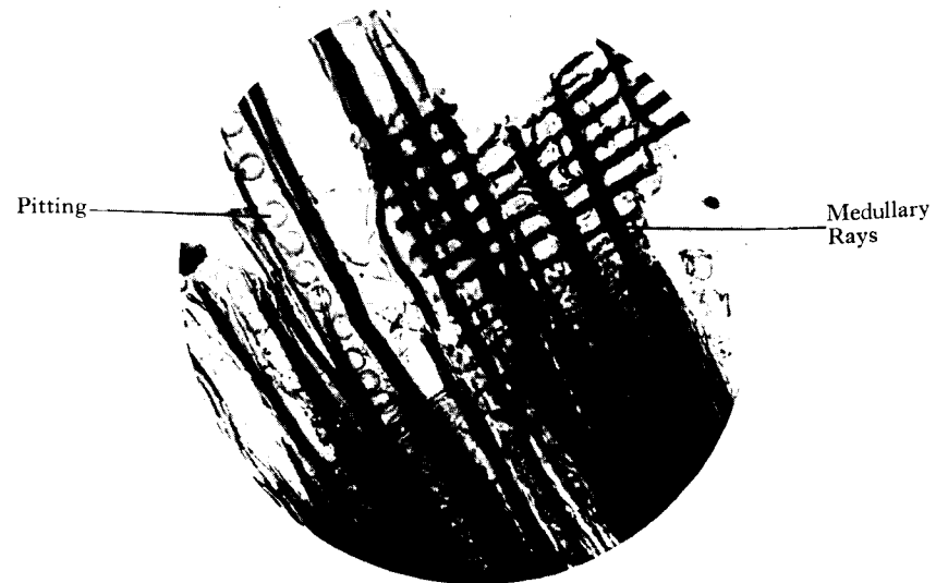
FIG. 15. Photomicrograph of maceration of sawdust from teeth of saw (showing the characteristic medullary ray and pitting of pine)
