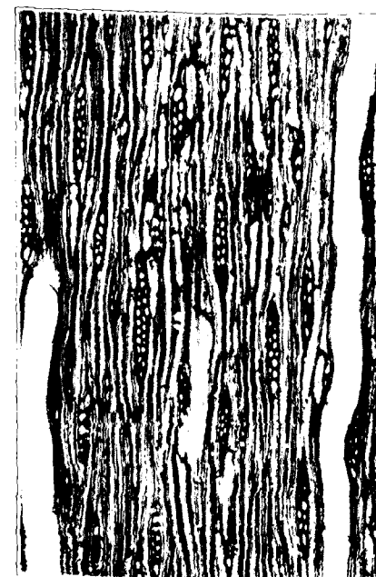
FIG. 3. Santalum austro-caledonicum . Tangential section, \times 57 .
