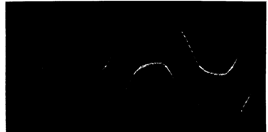
Plate 1. Current through coil a, machine running as a motor on no load.
