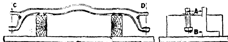
Two methods of testing the front axle for alignment.
